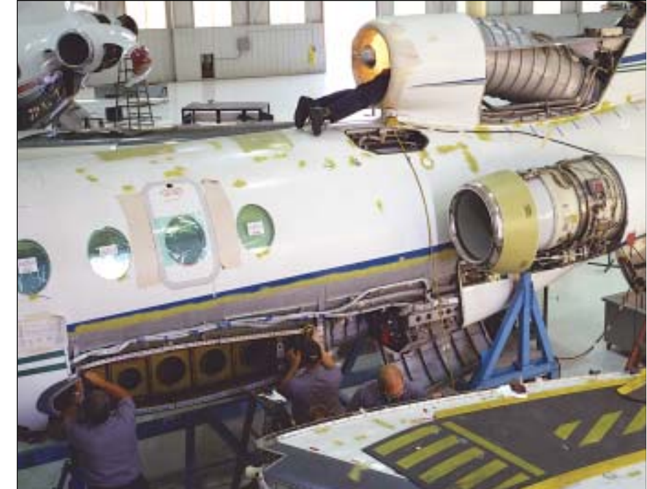
During an airframe inspection, corrosion was found on this Falcon 50. A wing demate was required to complete repairs.
