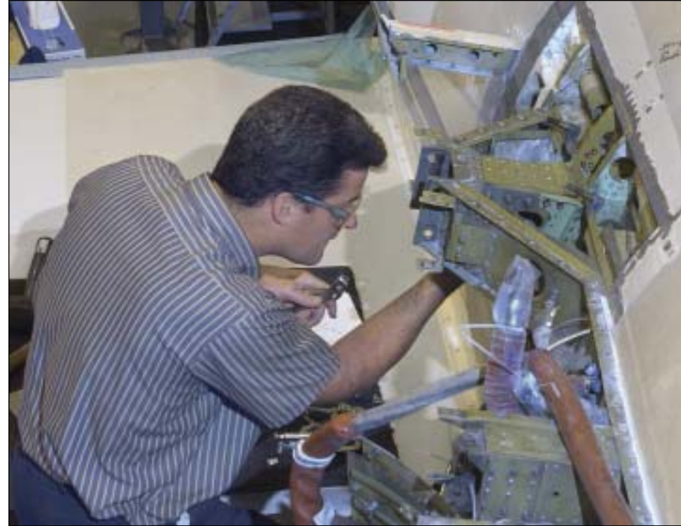
Tom Burke, a Duncan Aviation Airframe Structures Technician, completes a shear web modification on a Learjet 35.
